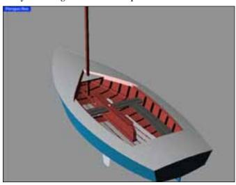
The 3-D model was then used to predict the equilibrium sinkage, trim, and righting moment for the boat with no additional flotation. As you can see, there is very little freeboard and waves would freely roll over the boat making it virtually impossible to bail out. In order to successfully bail out the boat and get
