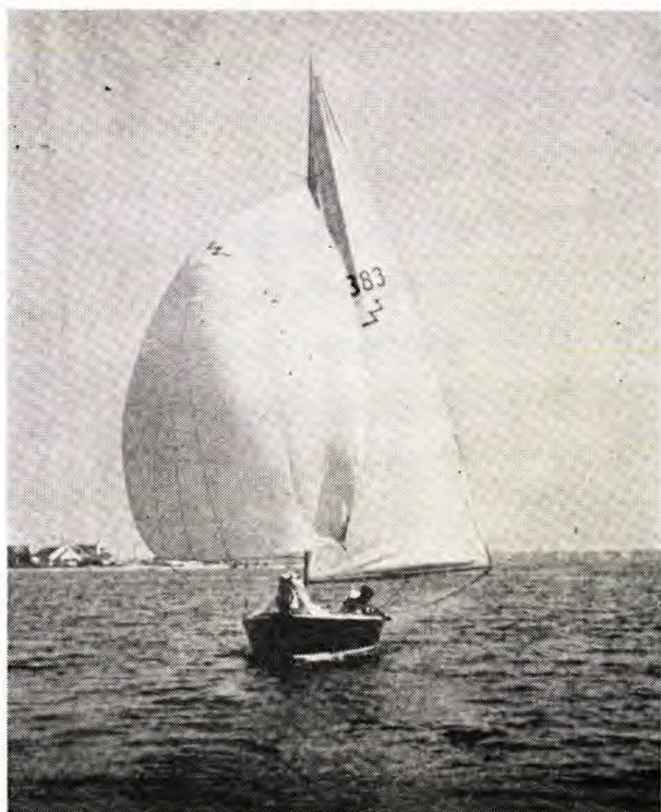
The spinnaker in a very light breeze. Pole attached to lower eye on mast; wind not sufficient to distend head of spinnaker; the slack mainsheet indicates lightness of breeze.
