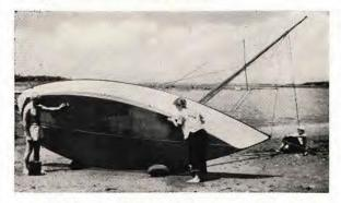
A Lightning has been hauled out, careened with two Airollers midships under the chine, while the crew cleans the bottom for the next race.
