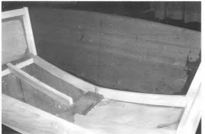
Forepeak framing above; transom framing, temporary flooring below.
