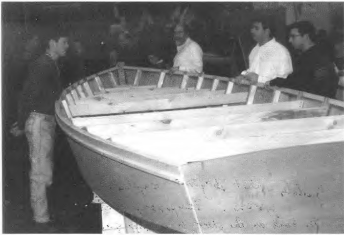
Builder Nat Bryant explaining the process. Note temporary cross-ties; the band on the sheer is a saw guide.
